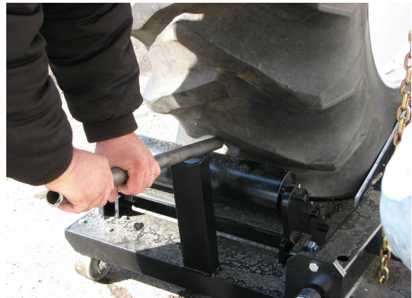
Figure 18. Rotating the wheel Rotating the wheel to align rim holes with the tapped holes in the hub or rim holes with captive lug studs.
